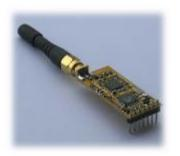
In the Arduino CanSat kit we are using APC220 which is a transceiver, with a highly versatile low power radio solution that is easy to setup and integrate into any project requiring a wireless RF link.
