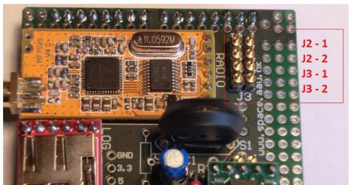
Figure 16: The CanSat Shield with radio
