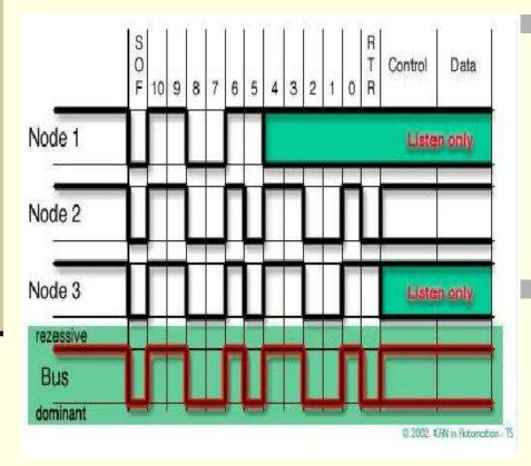
Access conflicts on the bus are resolved by a "wired and" mechanism, where the dominate state overwrites the recessive state.
