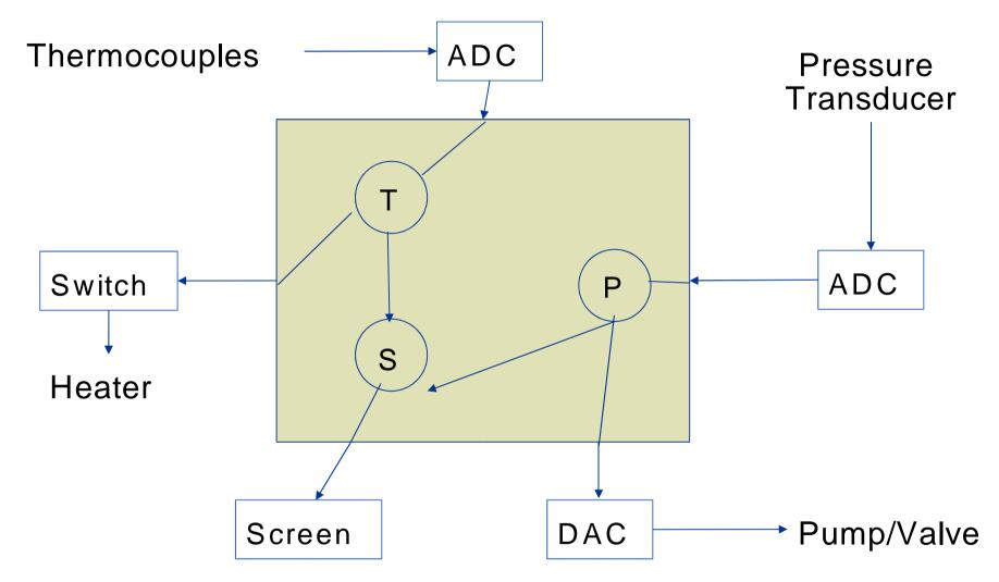
• Overall objective is to keep the temperature and pressure of some chemical process within well-defined limits
