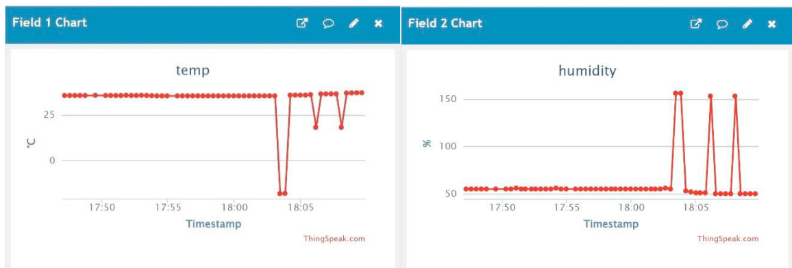
Fig. 6. Results of measurement data using ThingSpeak
